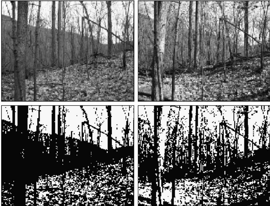
Fig. 4 – Two snapshots from the forest data set. Above: low resolution greyscale images; below: binary versions used for the blob analyses.
